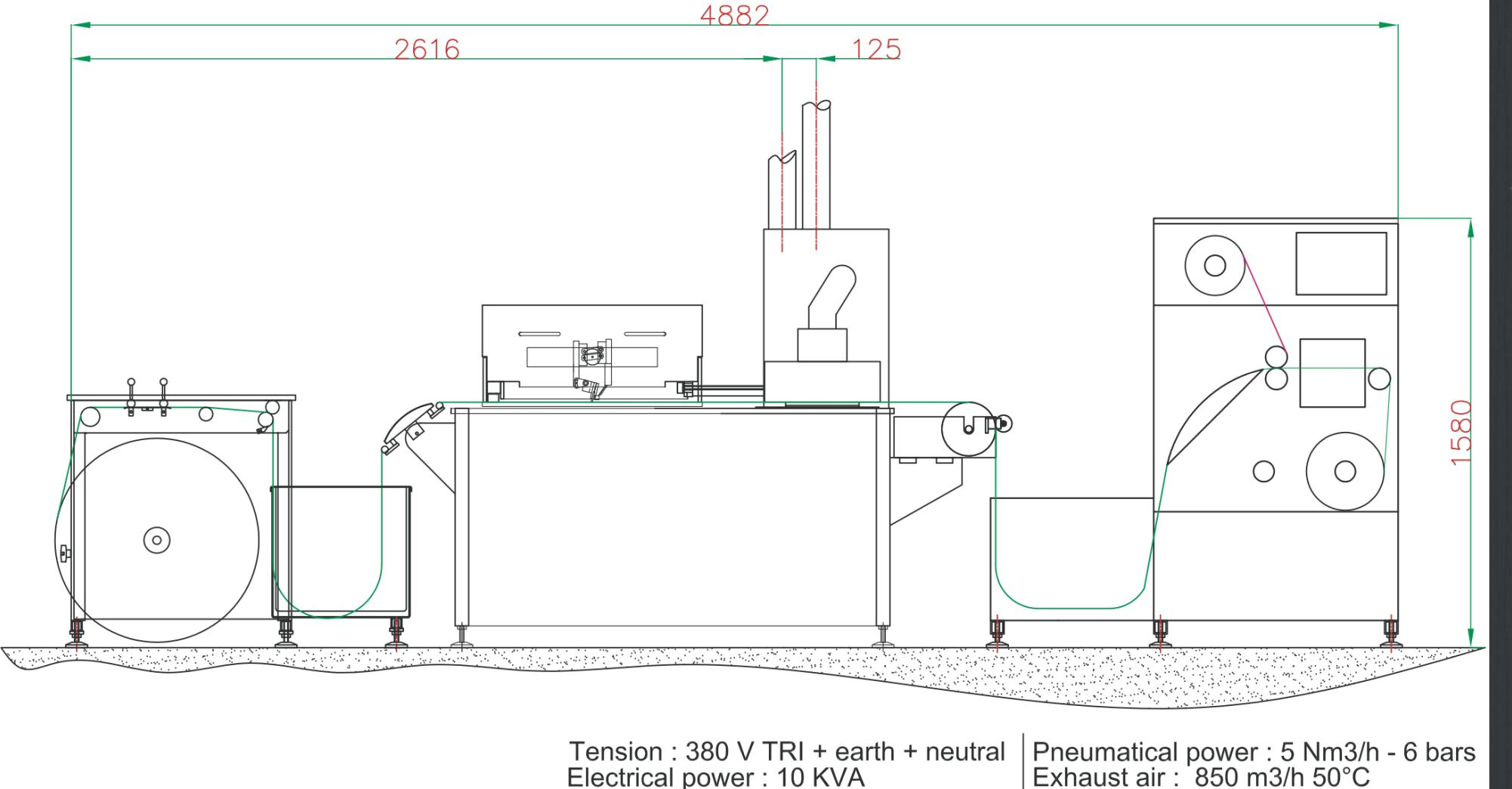
Tension : 380 V TRI + earth + neutral | Pneumatic power : 5 Nm3/h - 6 bars
